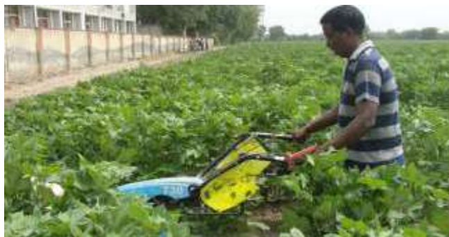
T2-YST attached to a rod on either side of wheels of a plough
