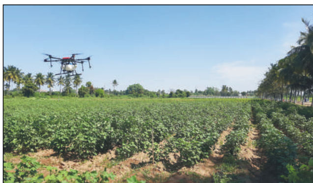
Fig no. 3.19.2 : Application of mepiquat chloride using chemical spraying drone
