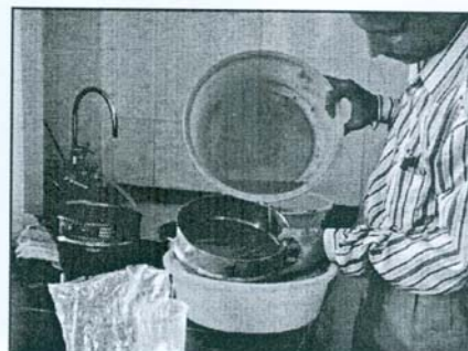
Suspension is passed through 100 mesh sieve
