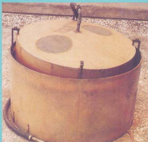
Batch Process Biogas Plant
